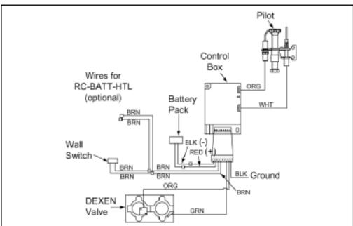
Figure 13 - "M" Series Intermittent Pilot Wiring Diagram
